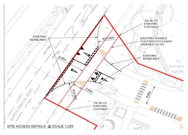
The initial design may need to be adjusted slightly through the S278 process to accommodate segregation of pedestrians and cyclists, however HCC is content that there is scope to do this if necessary and do not want to restrict the planning permission and are
